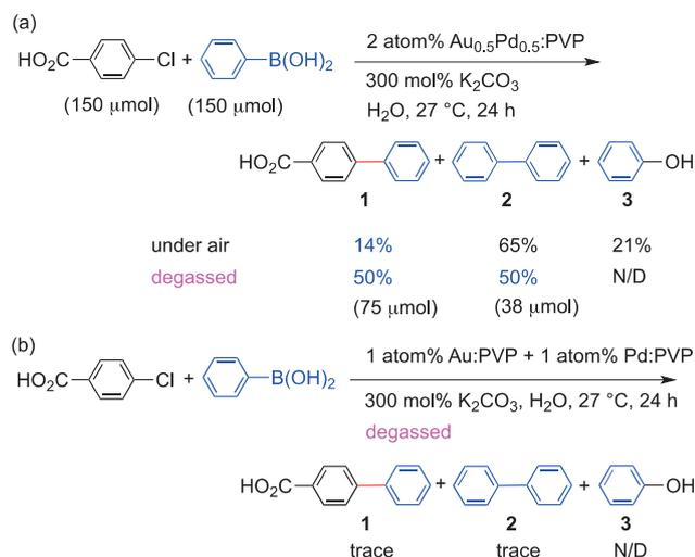
**Scheme 3.** Coupling reactions between CBA and PhB(OH)<sub>2</sub> catalyzed by (a) Au<sub>0.5</sub>Pd<sub>0.5</sub>:PVP and (b) Au:PVP + Pd:PVP.
