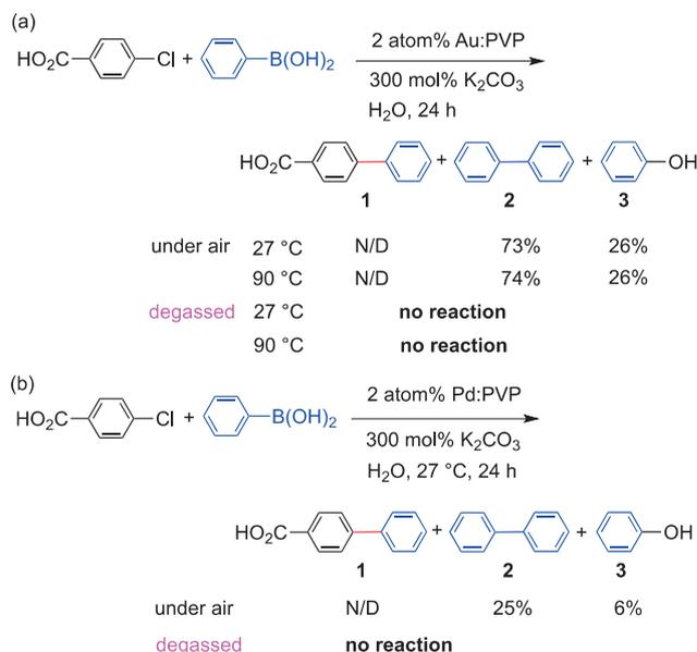
**Scheme 2.** Coupling reactions between CBA and PhB(OH)<sub>2</sub> catalyzed by (a) Au:PVP and (b) Pd:PVP, N/D: not detected.
