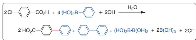
**Scheme 4.** The overall reaction catalyzed by Au<sub>0.5</sub>Pd<sub>0.5</sub>:PVP.
