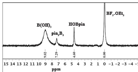
**Figure 1.** <sup>11</sup>B NMR spectra recorded at pH 9.7 in 33% D<sub>2</sub>O. Reaction conditions: CBA (0.15 mmol), PhBpin (0.15 mmol), 300 mol % K<sub>2</sub>CO<sub>3</sub>, 2 atom % Au<sub>0.5</sub>Pd<sub>0.5</sub>:PVP, 2 mL H<sub>2</sub>O, 1 mL D<sub>2</sub>O, 27 °C, 24 h degassed.
